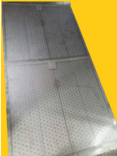
Single side inflated bulk milk cooler laser welded pillow plates
